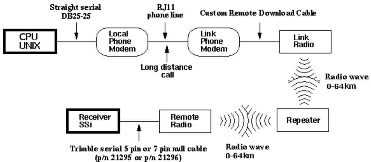
**NOTE:** The use of a repeater and directional antennas depends on the specifics of the site, distances signals need to travel, topography etc.
