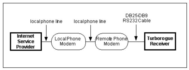
Trimble Receiver--Phone Modem--Phone Modem--PC
