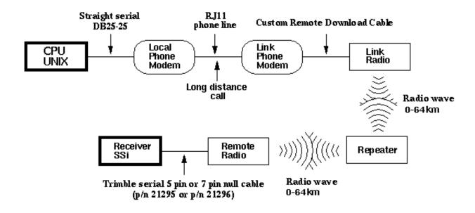
**NOTE:** The use of a repeater and directional antennas depends on the specifics of the site, distances signals need to travel, topography etc.
