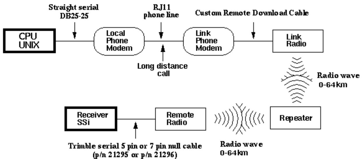
**NOTE:** The use of a repeater and directional antennas depends on the specifics of the site, distances signals need to travel, topography etc. Download rates will vary depending upon site location, local interference, phone line quality, and cellular service. Please contact Support ([support@unavco.org](mailto:support@unavco.org)) for more details.
