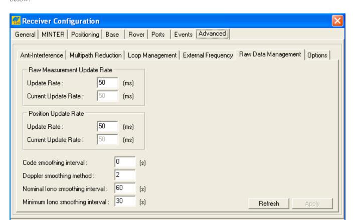
It is currently now possible to enable logging rates faster than 1 Hz from the front panel of the receiver. We have requested this capability of Topcon in a future firmware release.
