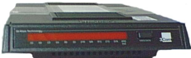
The Courier can connect at speeds up to 56 kbps on analog phone lines using x2 technology. It also provides full support for V.34+, V.34 standard, V.Fast Class, V.32 terbo and many other modulation schemes spanning the range of speeds between 300 bps to 56kbps. The Courier monitors line conditions and features carrier loss redial, remote configuration, error controls, data compression, and testing.
