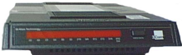
The Courier can connect at speeds up to 56 kbps on analog phone lines using x2 technology. It also provides full support for V.34+, V.34 standard, V.Fast Class, V.32 turbo and many other modulation schemes spanning the range of speeds between 300 bps to 56kbps. The Courier monitors line conditions and features carrier loss redial, remote configuration, error controls, data compression, and testing.
