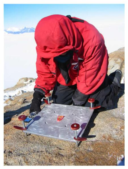
Eric Kendrick of Ohio State University works to install a mast using the custom jig on Moody Nunatak, Antarctica, as part of the WAGN network.
