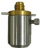
A 5/8" threaded leveling mount can be used, but we commonly use a simple non-leveling mount consisting of a stainless steel cup holding a brass adapter. The antenna is screwed onto the brass adapter and can be rotated to north. The adapter is then held in place in the cup with a set screw. The monument itself is installed as close to vertical as possible.
