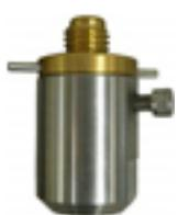
A 5/8" threaded leveling mount can be used, but we commonly use a simple non-leveling mount consisting of a stainless steel cup holding a brass adapter. The antenna is screwed onto the brass adapter and can be rotated to north. The adapter is then held in place in the cup with a set screw. The monument itself is installed as close to vertical as possible.
