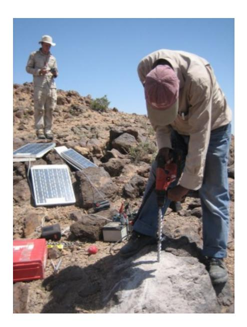
Feleke Worku of the Ethiopian Mapping Agency uses a battery-powered Hilti hammer drill to drill the hole for a monument pin in the Afar network.
