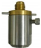
A 5/8" threaded leveling mount (cost \$150) can be used, but we commonly use a simple non-leveling mount consisting of a stainless steel cup holding a brass adapter. The antenna is screwed onto the brass adapter and can be rotated to north. The adapter is then held in place in the cup with a set screw. The monument itself is installed as close to vertical as possible.
