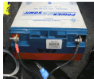
First Connect Battery. Ensure + Red, - Black!!!
