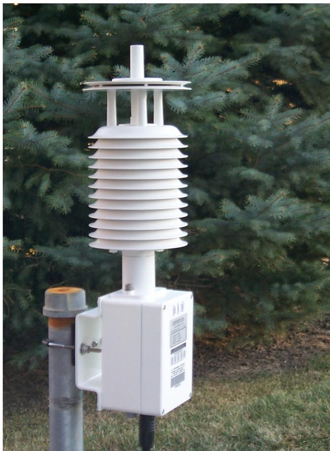
The Paroscientific MET3 Meteorological Measurement System measures barometric pressure, relative humidity, and temperature. The meteorological data is stored within the GPS data stream and can be extracted from the GPS data. The MET3 was one of three meteorological systems approved for use in the [SuomiNet GPS network](#). The table below shows the different receivers UNAVCO has used with the MET3. For more information on the MET3, see the [Paroscientific GPS Meteorology Support Site](#).
