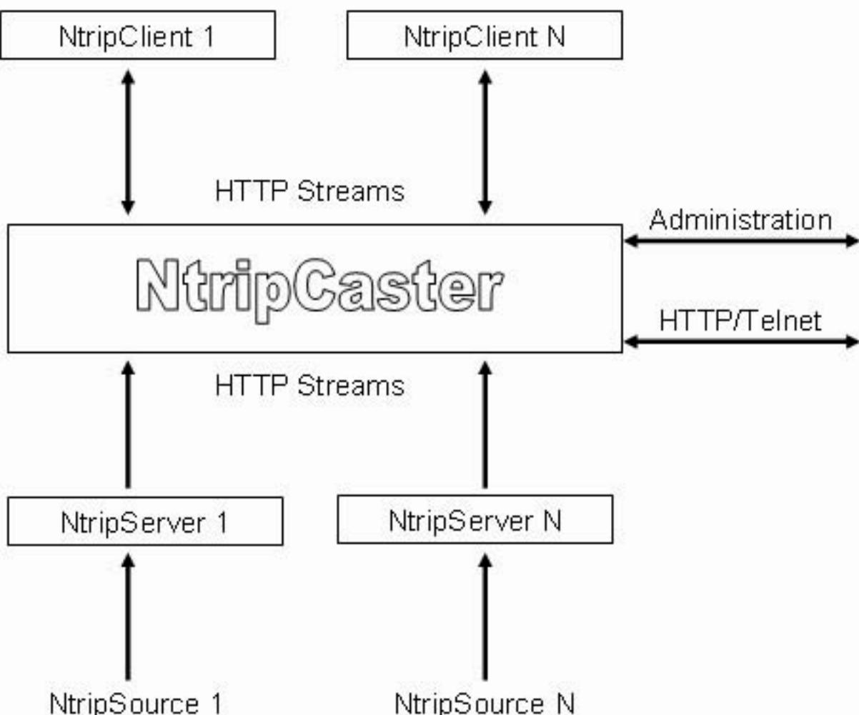
Figure 1: Schematic of a Ntrip network ([Trimble, 2004](#)).
