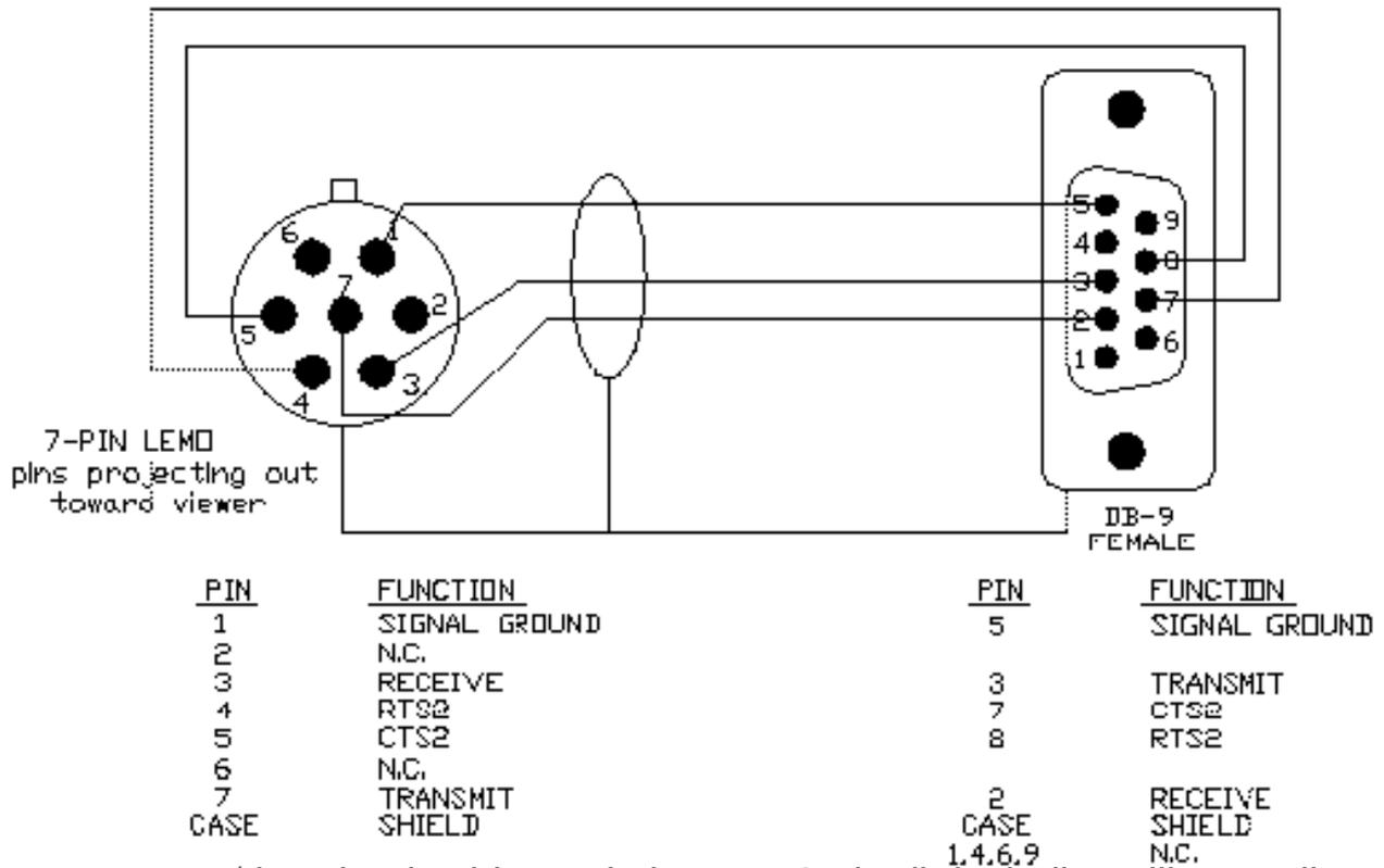
Battery power/download cable: 5-pin lemo to 9-pin db including alligator clip leads for powering a receiver.
