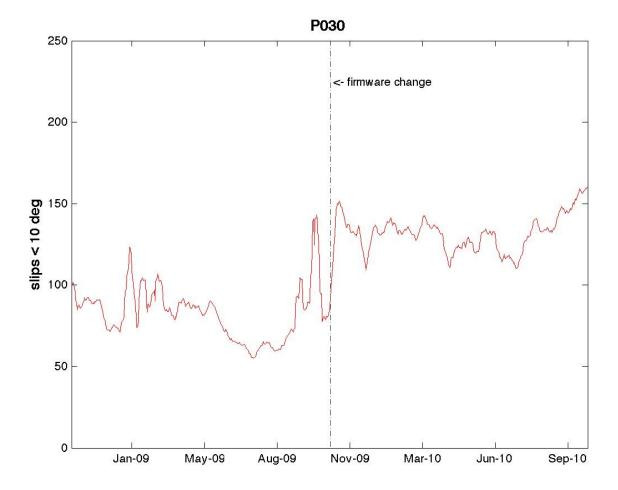
The following figure shows 24-hour totals of MP or IOD slips that occur at the site P030 when the elevation angles were > 10 degrees. The average number of IOD or MP slips before the firmware change is 2.34. The average IOD or MP slips after the firmware change is 4.90.
