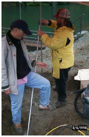
9. Repeat this process for the other 2 legs and insure they are spaced at 120 degrees off the north leg.
