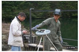
28. Place the top portion of the SCIGN adaptor onto the bottom portion of the adaptor. Use a Brunton compass to level the mount. To do this remove the set screws from beneath the bottom plate and adjust with an Allen wrench. When adjusted replace the setscrews.
