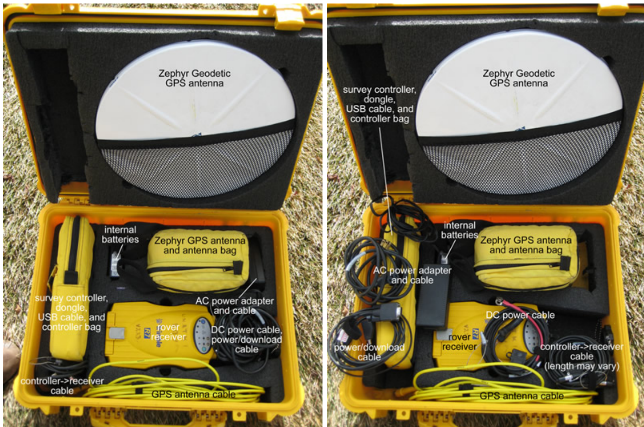
UNAVCO NSFEAR rover GPS unit: typical packing (left) and view of all components (right).
