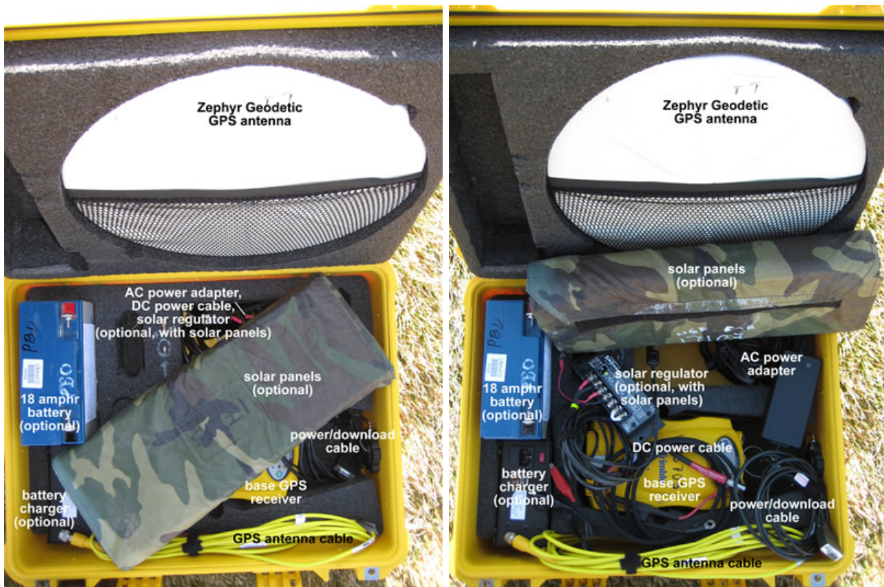
UNAVCO NSF EAR base GPS unit: typical packing (left) and view of all components (right).
