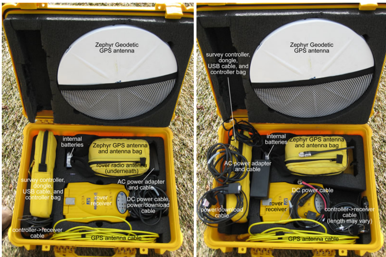
UNAVCO NSFEAR RTK rover GPS unit: typical packing (left) and view of all components (right).
