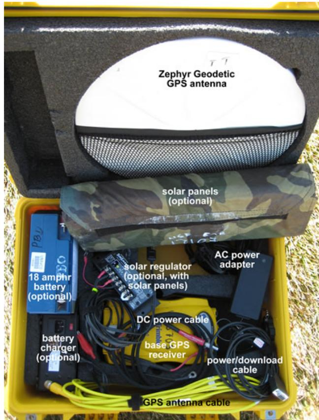
UNAVCO NSF EAR RTK base GPS unit: typical packing (left) and view of all components (right).
