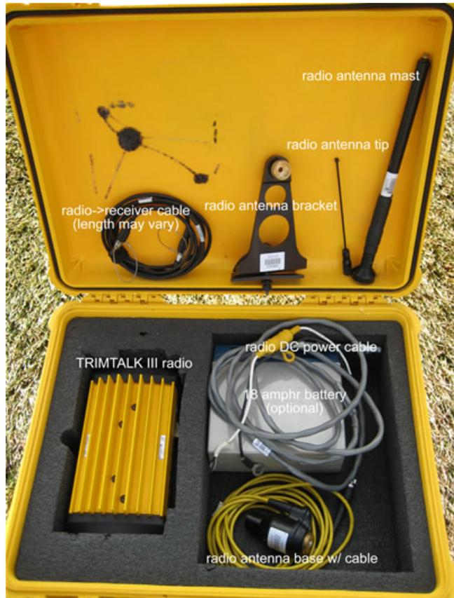
UNAVCO NSF EAR RTK base radio unit: typical packing (left) and view of all components (right).
