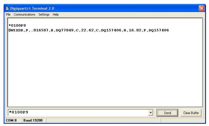
The P9 response is divided into a header and three measurement sections (pressure, temperature, and humidity). Each measurement consists of an identifier, a measurement value, a unit, and a transducer serial number separated by commas.
