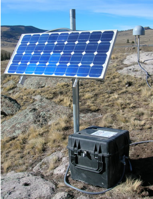
Pelican case enclosure as used in the Rio Grande network, Colorado and New Mexico.
