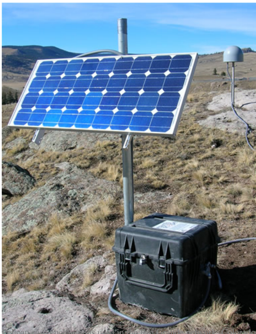
Pelican case and solar panel as used in the Red Rocks Assembly, Colorado and New Mexico.
