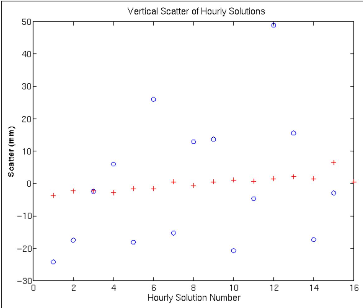
**Figure 2: Scatter of the baseline length of the hourly solutions for the two different zero baselines. The circles represent the individual hourly solutions of the Trimble 4000 SST and Trimble 4000 SSE mixed solutions. These solutions have an RMS of 19.3 millimeters. The plus marks are the individual solutions of the zero baseline with two Trimble 4000 SSI receivers. These solutions have an RMS of 2.1 millimeters.**
