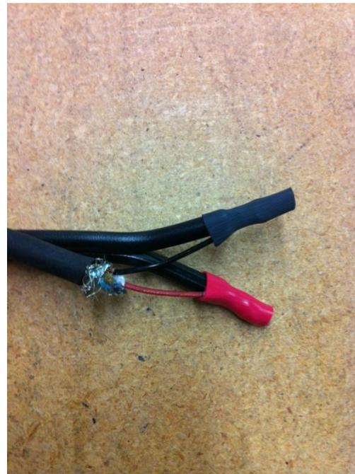
Now straighten the wire out and use another larger heat shrink sleeve to hold the two wires in place
