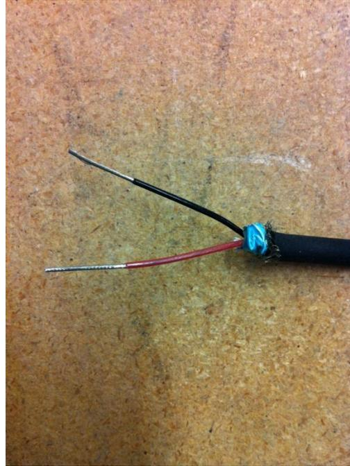
At this point the cable is ready to use, however I recommend adding an extra length of 16awg wire because the existing wires are quite small and short.
