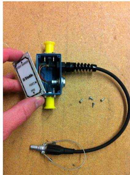
Next cut the wires inside the box as close to the female lemo plug as possible. This female lemo plug will not be used in the power cable but is quite an expensive item and could be used in another application in the future. Remove the black plastic nut inside the box to release the black cable, then unscrew and remove the two remaining black plastic pieces from the cable.
