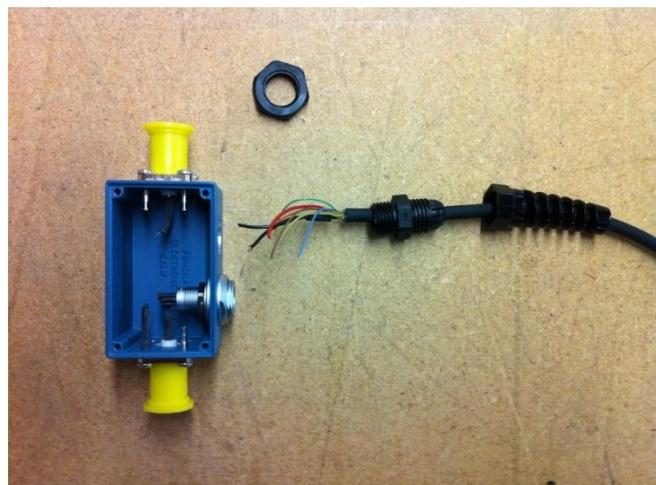
Trim off all of the extra wires from the black cable, leaving only the thicker Black(-) and Red(+) wires. You may need to strip a little more of the black cable to expose more of the two wires that we need.
