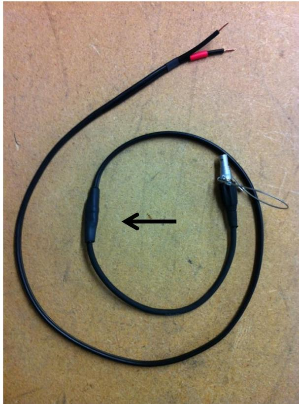
Make sure that you keep track of which wire is the positive(+). Once you have all of the heat shrink sleeves on, it is difficult to test. You can now use the female lemo plug to help with the testing, just plug it onto the top of the male lemo and use the exposed wires to test continuity. I also clearly mark which wire is positive(+) with another red heat shrink sleeve.
