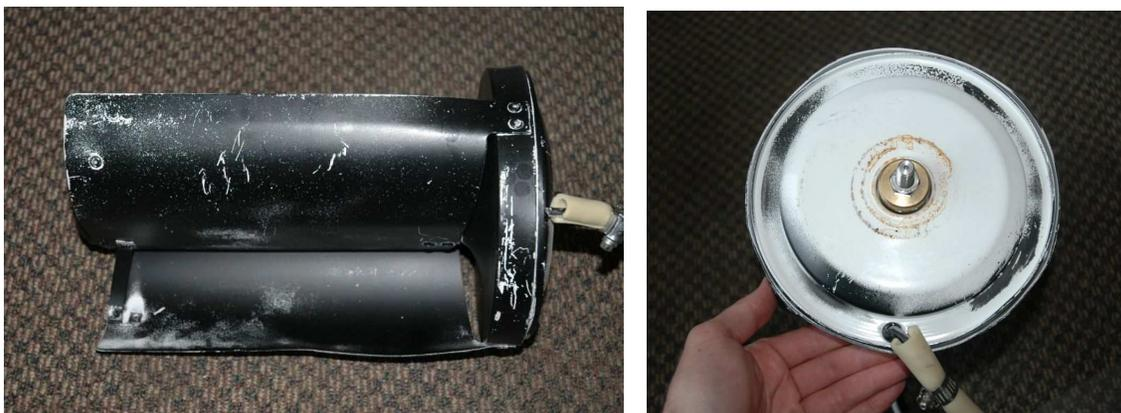
Figure 3. Forgen 500 Turbine Damage After Winter at Minna Bluff Antarctica.
