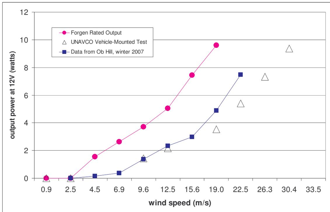
Figure 1. Forgen 500 output power at 12V.
