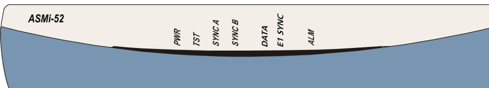
Figure 3-5. ASMi-52 Front Panel, E1 + DTE Serial Interface (4 Wire)
