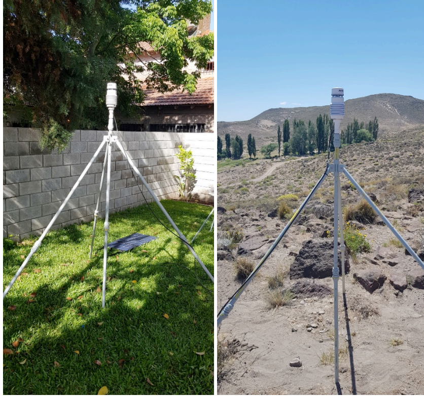
Figure 2. Airmar weather stations set up testing site and field deployment.
