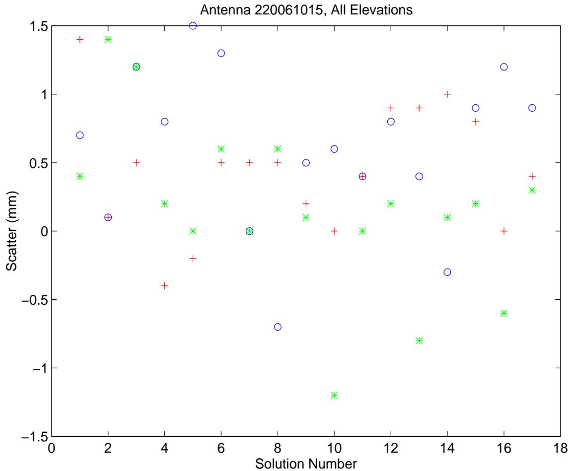
Figure 4: Height scatter for antenna 220061015. The blue “o” symbols represent solutions using a 10 degree elevation cutoff, the red “+” symbols use a 15 degree cutoff, the green “\*” symbols use a 20 degree cutoff. The scatter of these height solutions is the scatter about the mean of all the solutions. From this plot it appears as if the phase center does not vary as a function of elevation cutoff angle.
