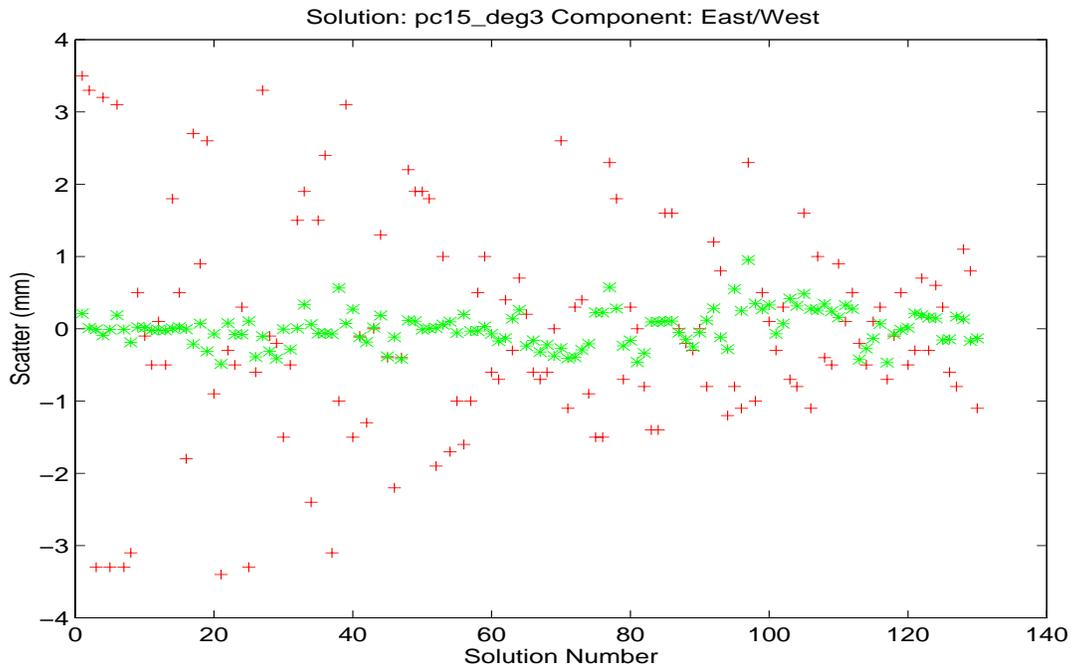
Figure 1: East/West baseline component scatter for antenna calibration tests. Red “+” symbols represent scatter without individual antenna phase offsets applied. Green “\*” symbols represent scatter of position residuals after estimation of individual phase offsets. Much of the high scatter is attributed to the rotation of antennas.
