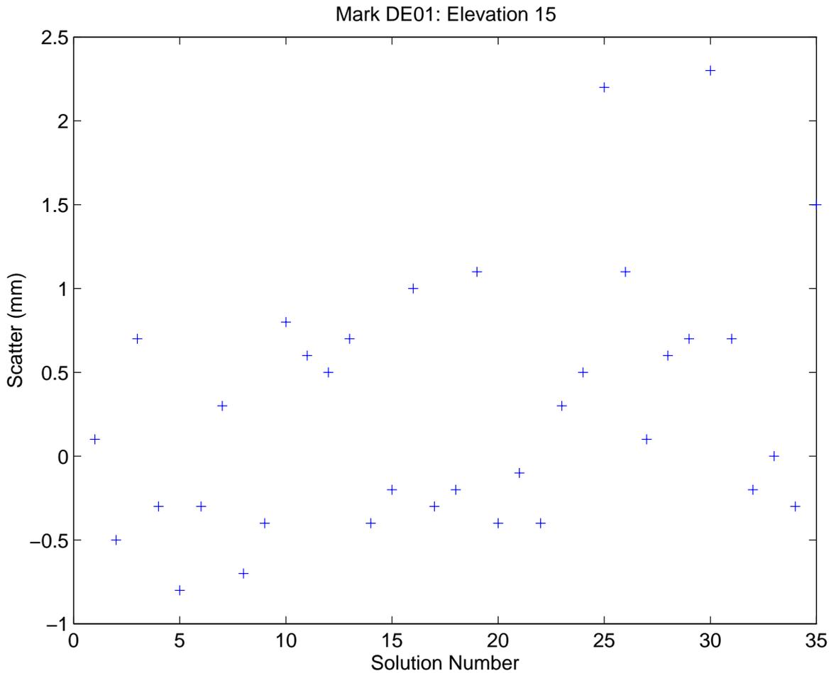
*Figure 3: Height scatter for baselines relative to mark DE01. For the first 16 solutions, antenna 220061014 was on the mark, the average of these solutions is 0.06mm. For the last 19 solutions, antenna 22062109 was on the mark, the average of these solutions is 0.5mm. From these baseline height solutions, it appears that the relative heights of the two antenna phase centers are within one mm of each other.*
