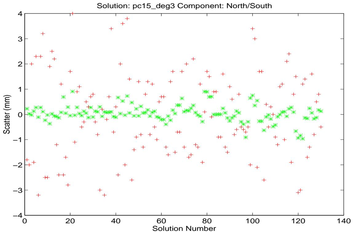
Figure 2: North/South baseline component scatter for antenna calibration tests. Red “+” symbols represent scatter without individual antenna phase offsets applied. Green “\*” symbols represent scatter of position residuals after estimation of individual phase offsets. Much of the high scatter is attributed to the rotation of antennas.
