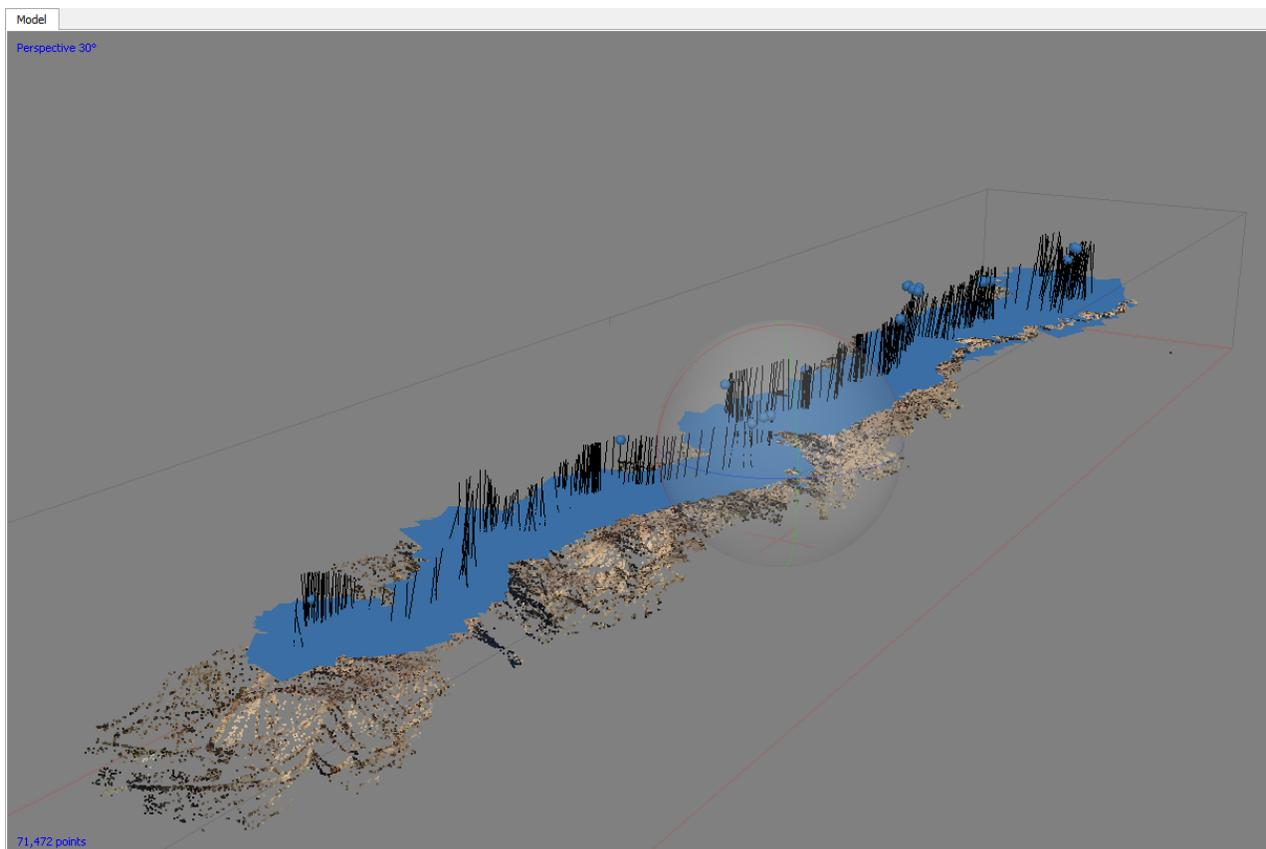
After the photos are aligned, a sparse point cloud will appear with blue rectangles indicating each camera position.
