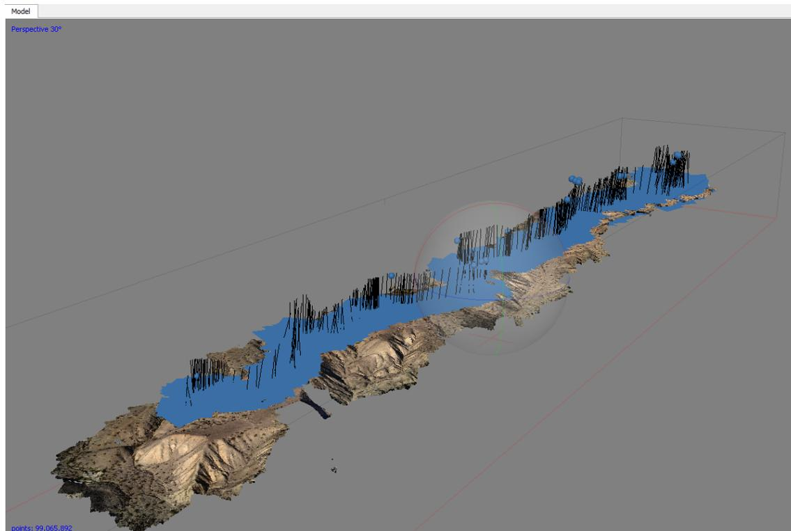
The dense point cloud operation fills in all the blank or empty areas in the sparse cloud.
