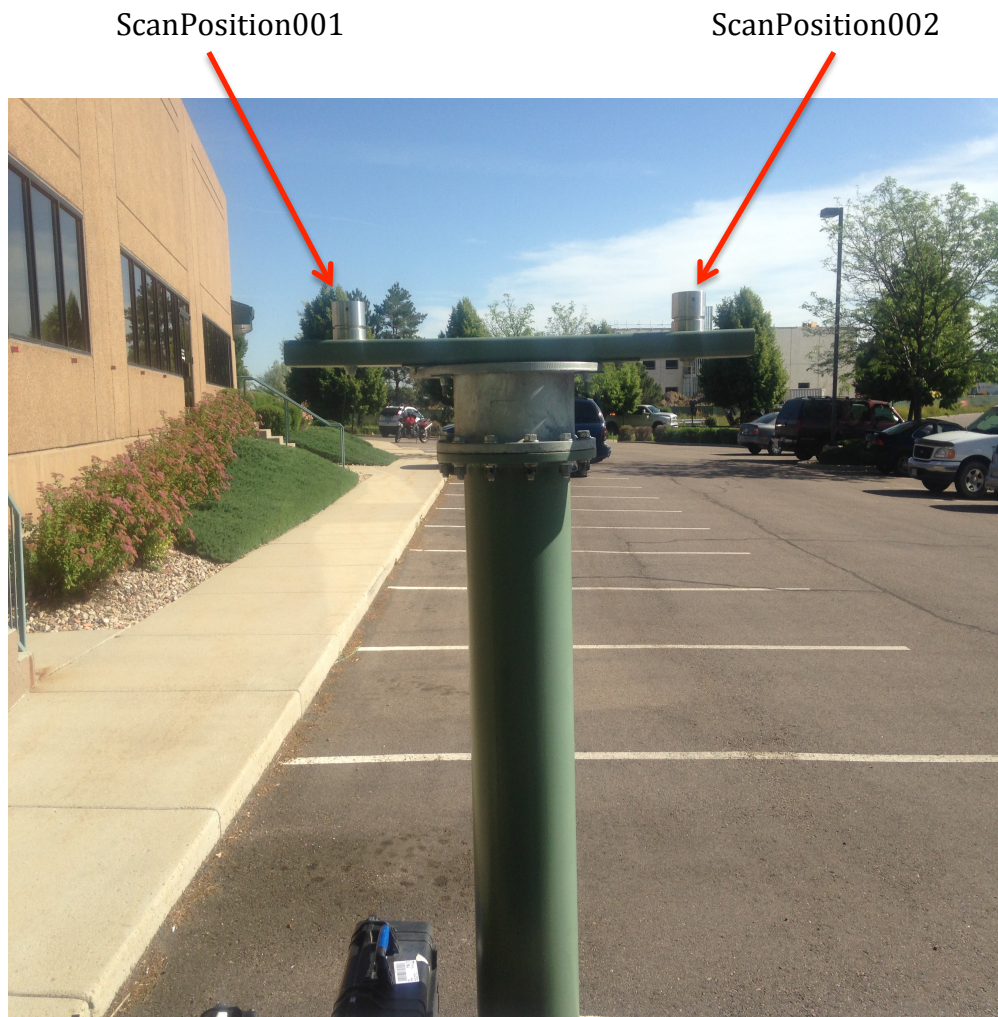
Figure 1 This is the dual position TLS mount. Scans are performed from ScanPosition001 and then ScanPostion002.
