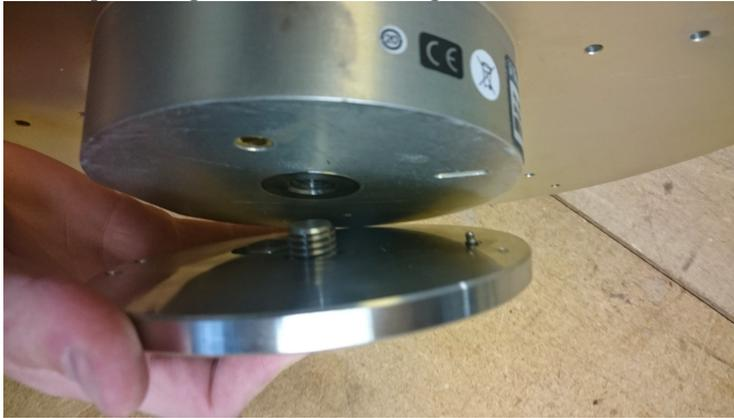
5. Reattach the antenna and top plate to the bottom plat by using the 7/32 wrench. Make sure both bottom and top N engravings match up.
