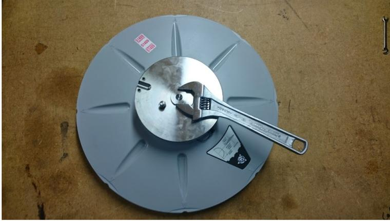
4. Screw the top plate onto the choke ring, and match up the security pin with corresponding slot in choke ring.
