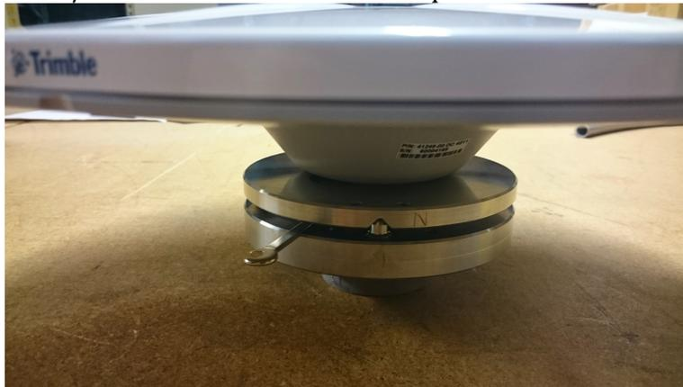
3. Now that the antenna is free, use an adjustable wrench to remove top SCIGN plate from the antenna.
