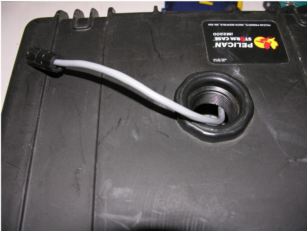
Route power plug outside of case for use. Move inside for travel and replace plug.
