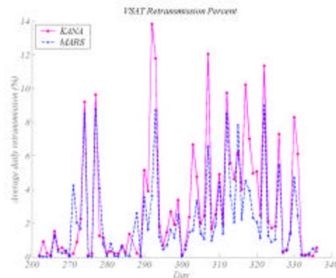
**Figure 10. The percent of retransmissions calculated as a daily average. High retransmissions correlate with periods of data outage (Figure 9). The remaining retransmission requests are for data housekeeping at the hub.**
