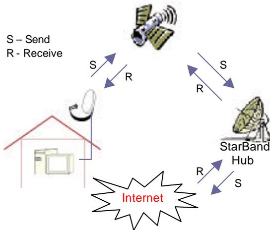
**Figure 2. The StarBand VSAT network currently provides two-way Internet service within the coterminous US with planned coverage for Alaska, Hawaii, and Mexico. Data are routed from a remote user to either GE-4 or the Telstar 7 satellite to the StarBand hub, which has a direct link to the Internet.**
