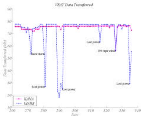
**Figure 9. Data (in Mb) transmitted from the MARS and KANA remote sites. Significant periods of data loss are labeled and explained in the text.**
