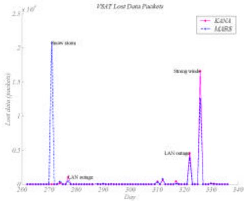
**Figure 11. Lost data packets not attributable to power outages. Significant periods of data loss are labeled and explained in the text.**
