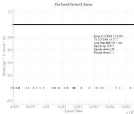
**Figure 4. Ping statistics indicate a 1.1% downtime for the StarBand network connection over a 10-day period. A value of 1 indicates the network was operational. A value of zero means the remote was out of contact.**
