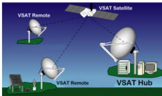
**Figure 1. A typical VSAT network depicting two-way communications from remote terminals through a VSAT satellite to a central hub.**
