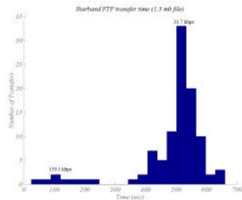
**Figure 3. FTP transfer time in seconds for a 1.5 Mb file from a remote station. Bimodal distributions of transfer times indicate burst transfer speeds of 159 kbps and sustained uplink speeds of 32 kbps.**
