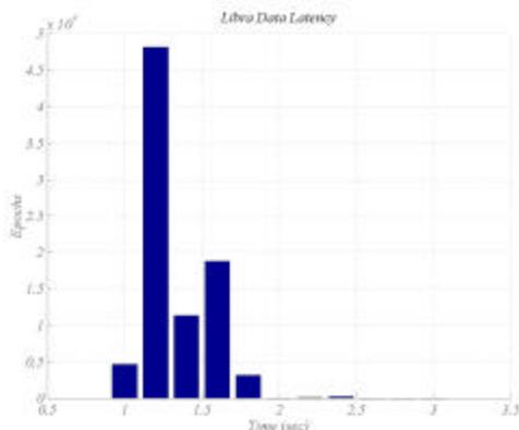
**Figure 12. Latency values for 1 second GPS data from station MARS for a 24-hour period. Note that the majority of data packets arrive within 1.2 seconds.**
