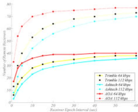
**Figure 7. A simulation of the number of remote stations possible given either 64 or 112 kbps throughput for a range of streamed data types. For this calculation a hub overhead factor of 8000 bps, a frame length of 5 s, a transmission overhead gap of .072 s and a packet size of 2584 bits were assumed.**
