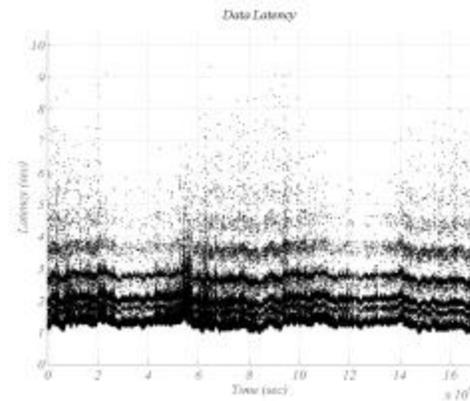
**Figure 5. Plot of data latency in seconds versus time for a 48-hour period. Data latency vary over a range of 1-10 s and with periods of high data latency corresponding to periods of high user activity on the StarBand network.**
