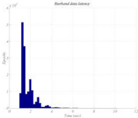
**Figure 6. Latency data from Figure 5 plotted as a latency histogram. Note that a majority of the data packets arrive within 4 seconds.**
