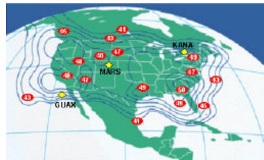
**Figure 8. Coverage area for the GE-1 satellite showing contours of equal EIRP. Station MARS and KANA were used in this evaluation. Station GUAX is an operational station deployed since the evaluation.**
