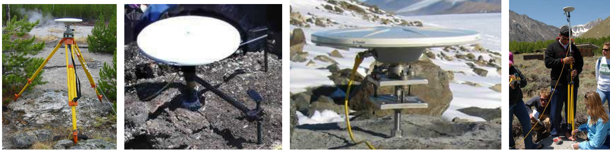
Figure 8: Examples of antenna mounts. (a) Standard tripods are bulky but are ideal for sites where the antenna must be elevated. (b) Fixed-height spike mounts are lightweight and highly portable; good for remote, open areas. (c) Fixed-height leveling mounts screw directly onto a threaded pin monument; highly portable and highly stable. (d) Bipods can be used for fast-static occupations or, by removing the legs, for kinematic surveys. Ideal for surveys with many survey marks within a small area.
