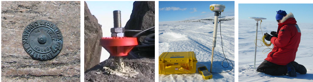
Figure 7: Examples of benchmarks. (a) A circular marker at the bedrock surface, with a pin which extends and anchors it into the rock. This mark requires a tripod, bipod, or spike mount setup (see below). Another common design is a stainless steel pin epoxied into bedrock, flush with the rock surface. (b) A threaded, stainless steel pin epoxied into bedrock. Often a tripod, bipod, or spike mount setup can be used, although a leveling mount can be screwed directly onto the pin for a low-profile, stable option suitable for both short- and long-term deployments. (c) Bamboo frozen into glacier ice, shown here with the antenna mounted on a PVC sleeve which slides over the bamboo. (d) A metal rod pushed into compact snow on an ice stream, suitable for long-term deployments.
