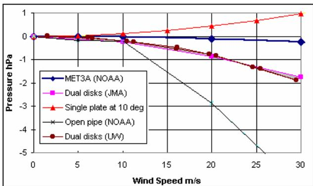
Figure 7. Wind-Induced Errors on Pressure Readings
