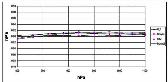
Figure 5. Barometer Repeatability, Hysteresis and Linearity
