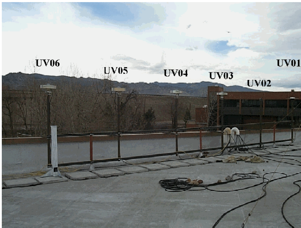
Figure 2-1: Benchmark location and antenna mounting system on the roof of the UNAVCO building. An Ashtech ZXII with antenna ASH700936A_M was run on benchmark UV06 during the entire testing phase. Benchmark UV05 was used for all zero baseline testing while UV04 and UV03 were used for short baseline tests. Benchmarks UV02 and UV01 were not used.
