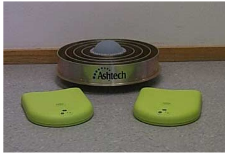
Figure 2-5: Javad Positioning Systems Legacy receiver with ASH701945.02B Ashtech Choke Ring antenna.
