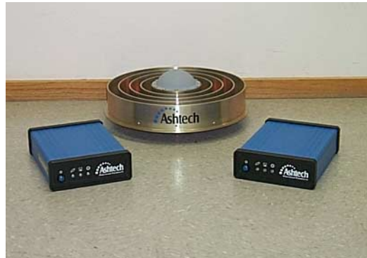
Figure 2-3: Ashtech u-Z GPS receiver with Ashtech ASH701945.02B Choke Ring antenna.
