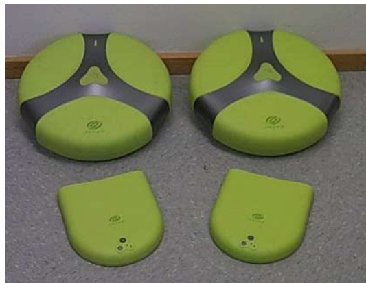
Figure 2-4: Javad Positioning Systems Legacy receiver with JPS Regant DD E (Dual Depth Choke Ring) antenna. The Legacy receiver was also tested with the JPS Regant SD E (Single Depth Choke Ring) antenna (not shown)
