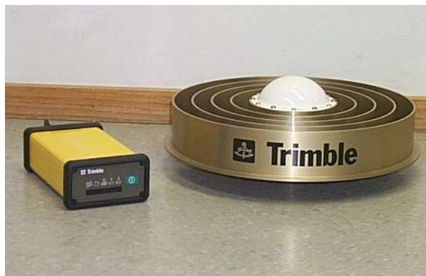
Figure 2-7: Trimble 4700 with TRM29659.00 Trimble Choke Ring antenna.
