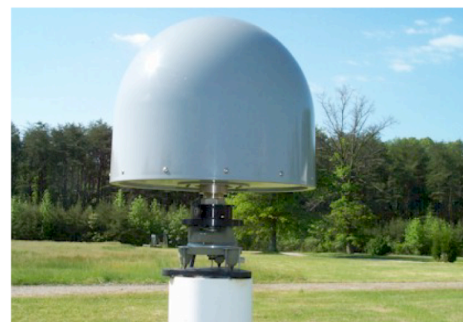
Figure 18: Antenna models used in the 205 km baseline between PIN2 and GOLD.
