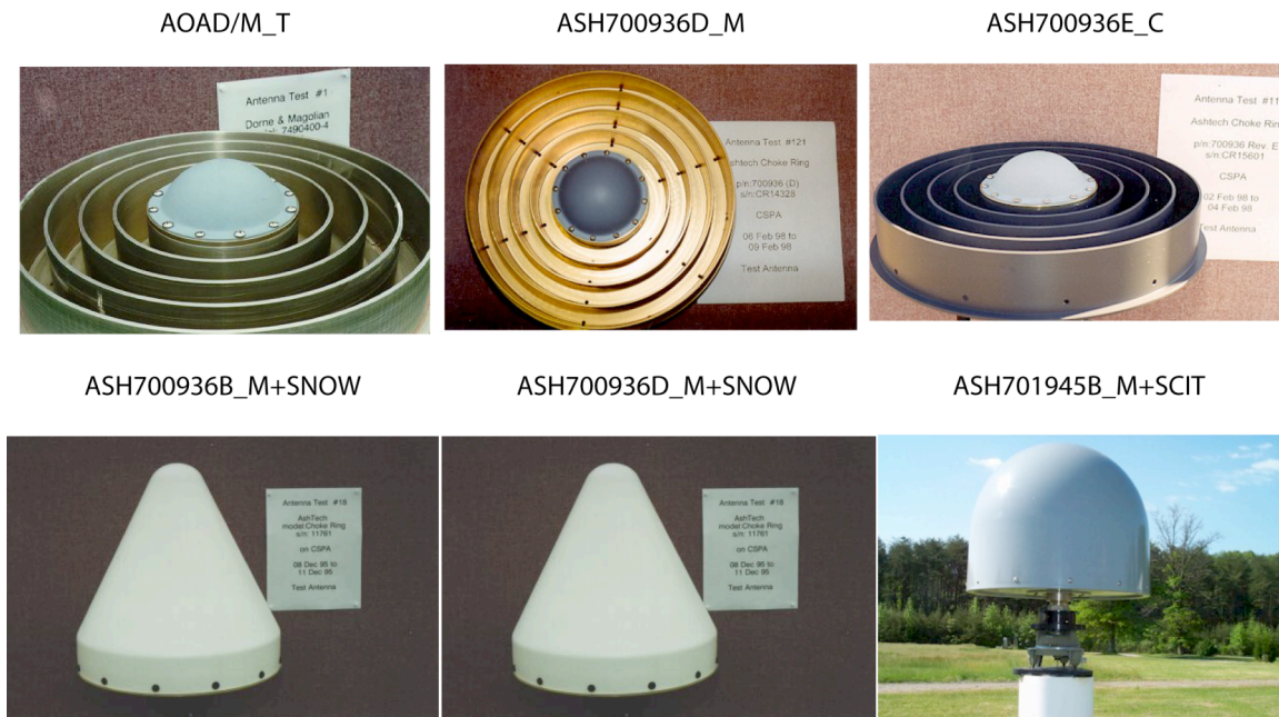
Figure 2: Antennas used in this experiment. All figures downloaded from the NGS phase center calibration page 3 .
