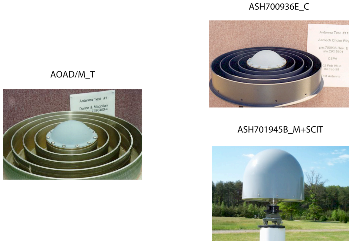
Figure 6: Antenna models used in the 50 meter baseline between PIN2 and PIN1.
