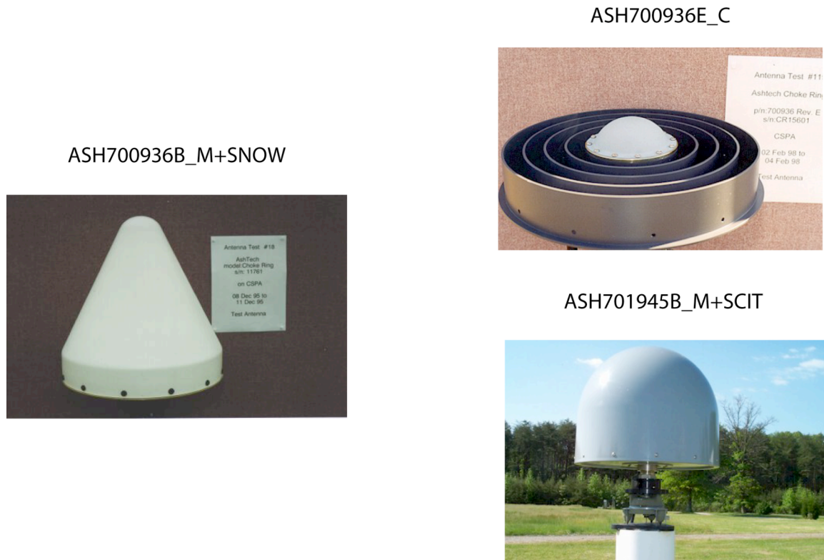
Figure 15: Antenna models used in the 32 km baseline between PIN2 and WIDC.
