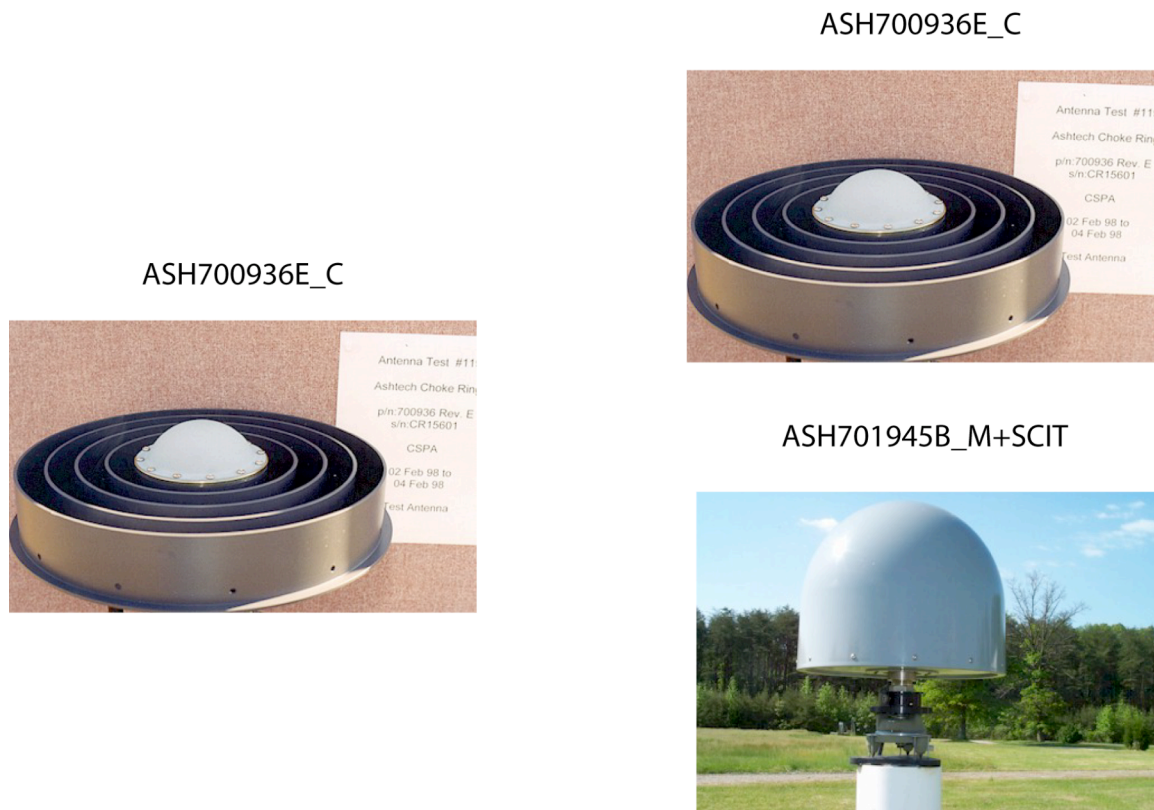
Figure 9: Antenna models used in the 72 km baseline between PIN2 and PPBF. This baseline is the only one in the test where the antenna model was the same at both stations.
