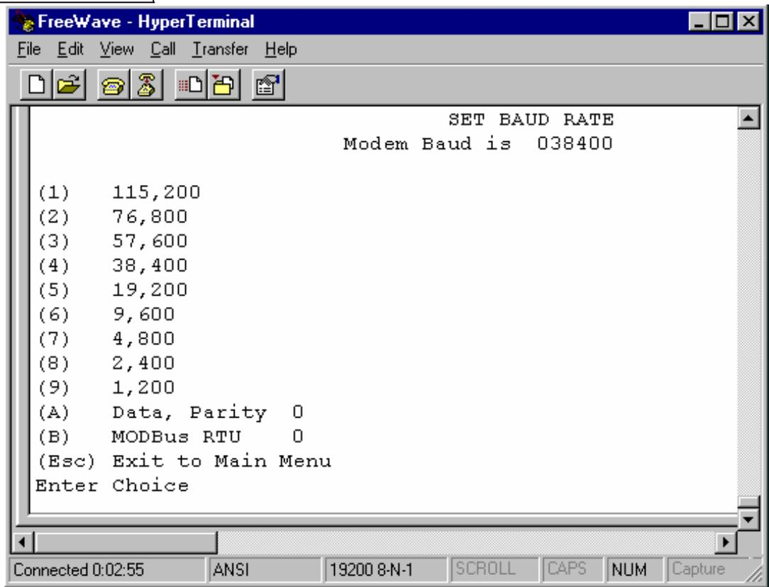
The Baud Rate section of the user interface provides two other important parameters, the ability to change the transceiver's word length and to put it into ModBus RTU mode.
