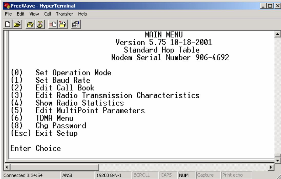
The initial menu provides the Transceiver's unique serial number, firmware version, and the set of choices for editing the operational parameters and viewing the performance data.
