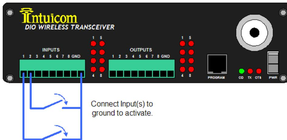
**Figure 6-1: Input Connection - Simple Contact Closure**
