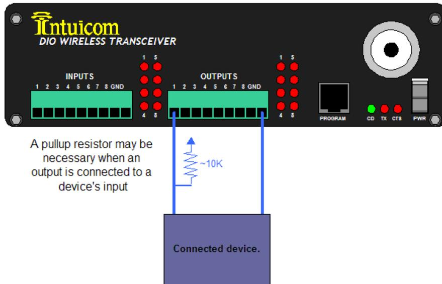
Figure 7-2: Output Connection - Device with Pullup Resistor
