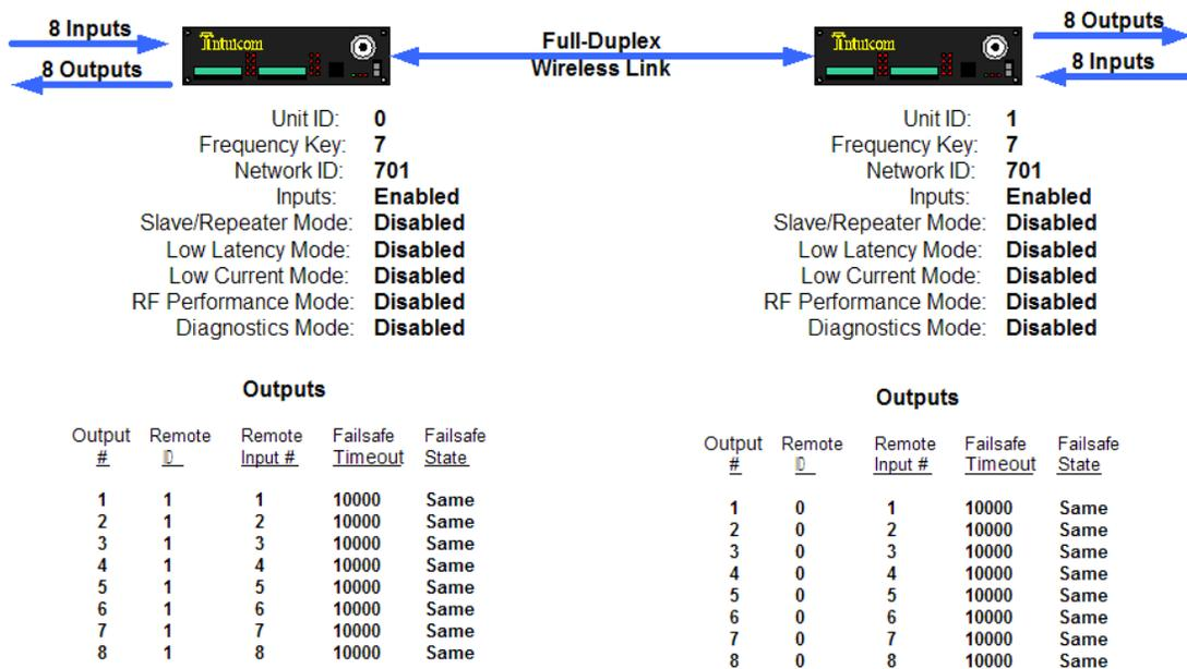
Figure 9-4: CommPro - Example DIO Network Configuration
