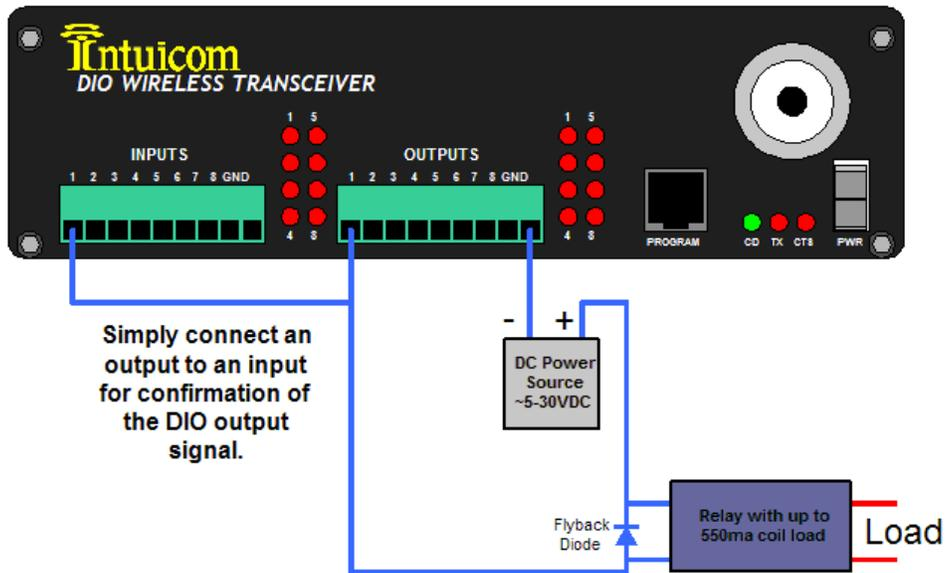
Figure 7-3: Output Connection - Relay with Confirmation
