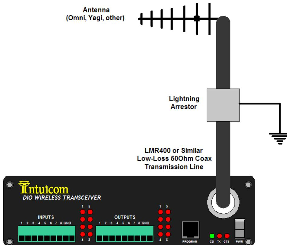
**Figure 8-1: Antenna Connection**
