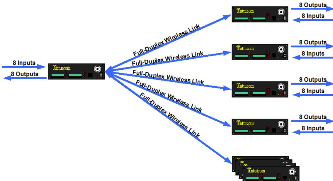
Figure 2-2: Point to Multipoint Network Architecture
