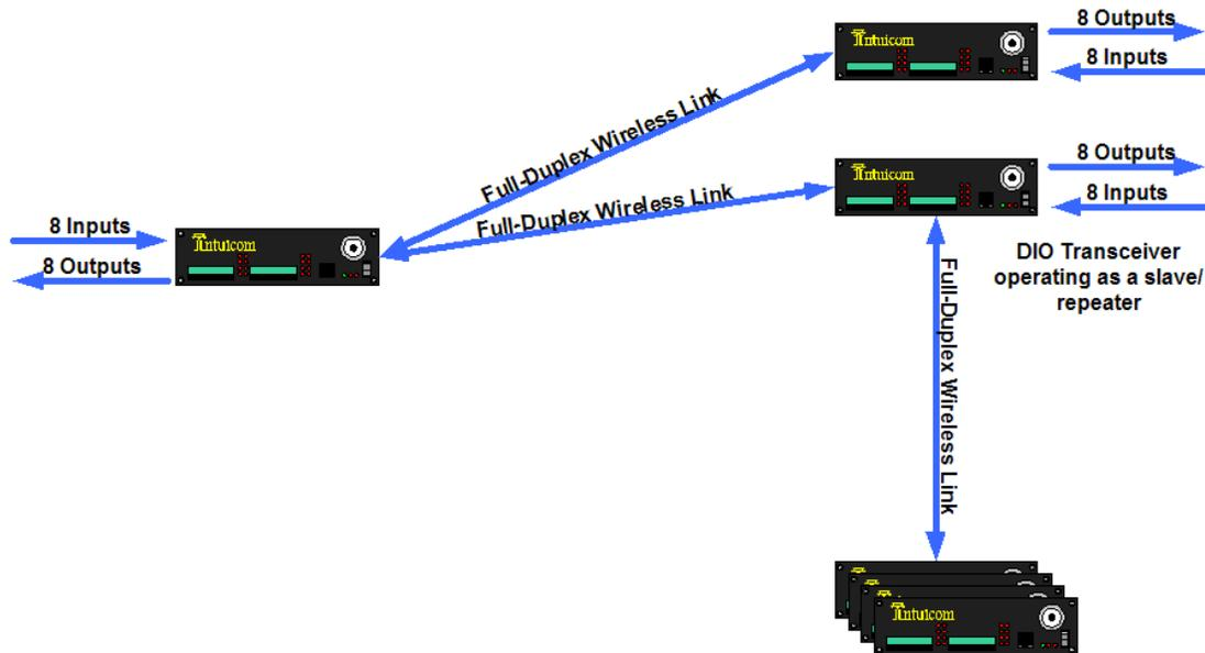
**Figure 2-3: Point to Multipoint with Repeater**
