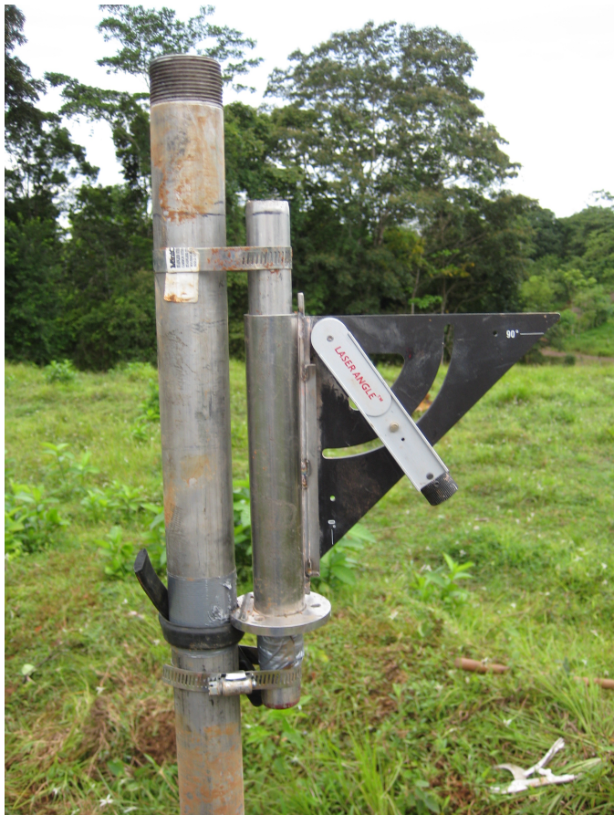
Figure 3 – For this particular monument, 1.25" pipe was used instead of solid steel rod. The laser jig was attached to the side of the center pipe with hose clamps.
