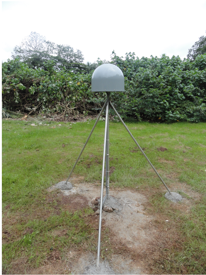
Figure 4 – A finished hand augered monument. Each leg extends 5 feet below ground level.
