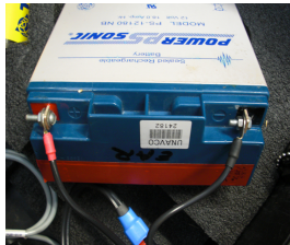
First Connect Battery. Ensure + Red, - Black!!!
