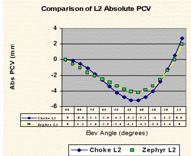
It can be seen that the absolute L1 phase center variation is significantly larger for the choke ring than for the Zephyr Geodetic Antenna. The L2 response is approximately the same for both antennas, within about 1-2mm.
