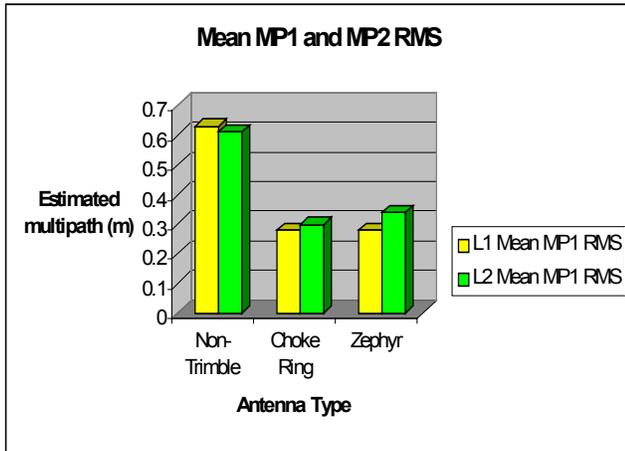
The non-Trimble conventional antenna design results contained approximately twice the levels of L1 and L2 multipath than those seen in both the choke ring and Zephyr antennas, in this large data sample of more than half a million measurements.
