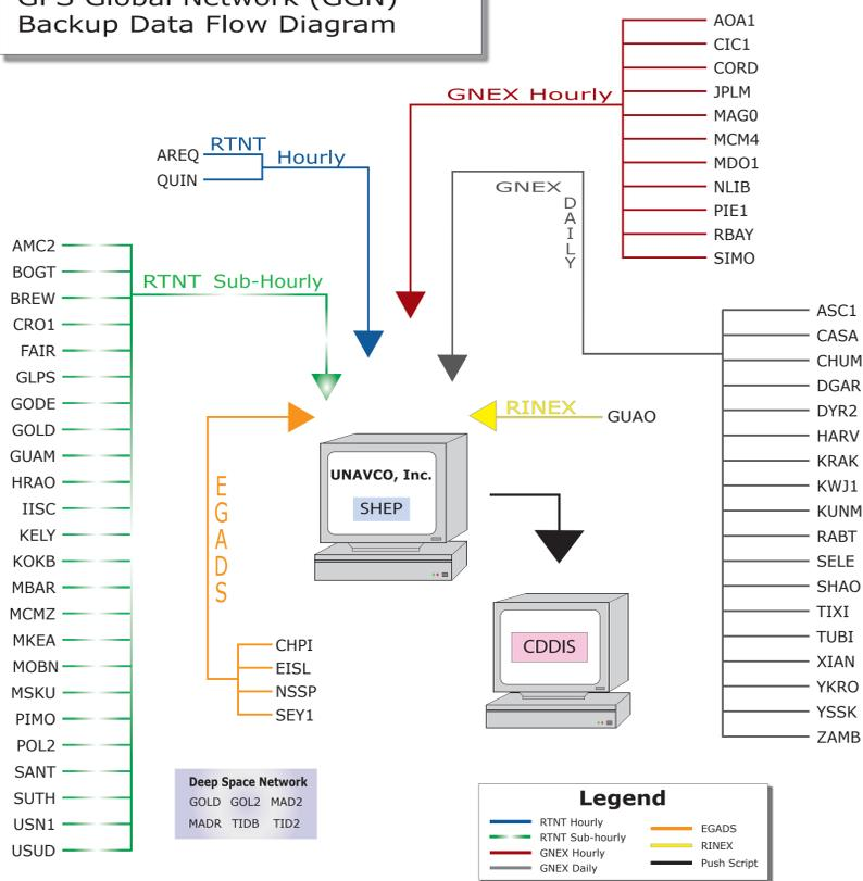
Schematic representation of UNAVCO backup operations of JPL data transfers. UNAVCO maintains a continuous readiness to provide data backup of JPL functions in case of an outage in JPL operations. The backup functions include data retrieval, RINEX conversion, data archiving, and data forwarding to the CDDIS of regular IGS products. In addition, normal station troubleshooting and maintenance tasks are provided during outages.
