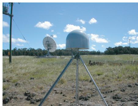
The newly erected SCIGN stainless steel, short drill-braced monument on Easter Island (ISPA). The new station runs an Ashtech MicroZ receiver with Ashtech Choke Ring Antenna and Tall SCIGN Radome. The station also includes a MET pack for meteorological measurements. Station uses a Linux computer and shares VSAT data communications routing with IRIS Seismic station.
