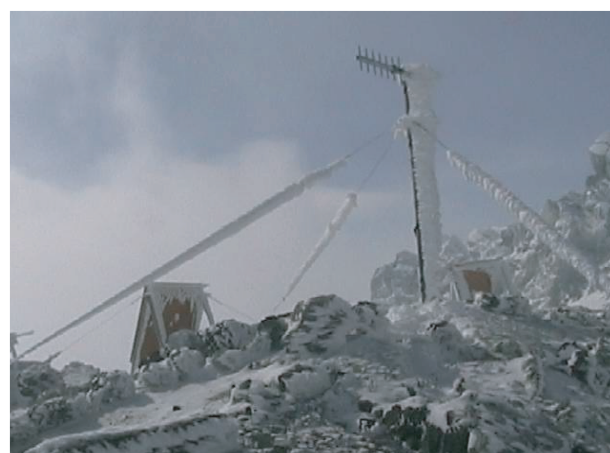
Rime icing at a Mt. Erebus site. Environmental sensor data indicated similar icing was likely just after 2003.05.
