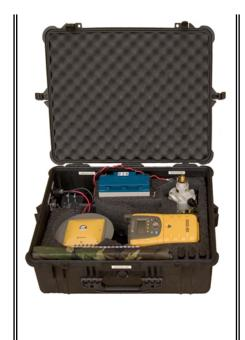
NSF's EarthScope Science panel. The systems have been designed for stand-alone temporary or semi-permanent deployment that will be used for densifying areas not sufficiently covered by continuous GPS and for responding to volcanic and tectonic crises. Six of the 100 systems are equipped with realtime kinematic (RTK) capability for such uses as rapid fault mapping and GIS-based geologic mapping. For <u>EarthScope</u> campaigns only. Antenna mounts must be requested separately.
