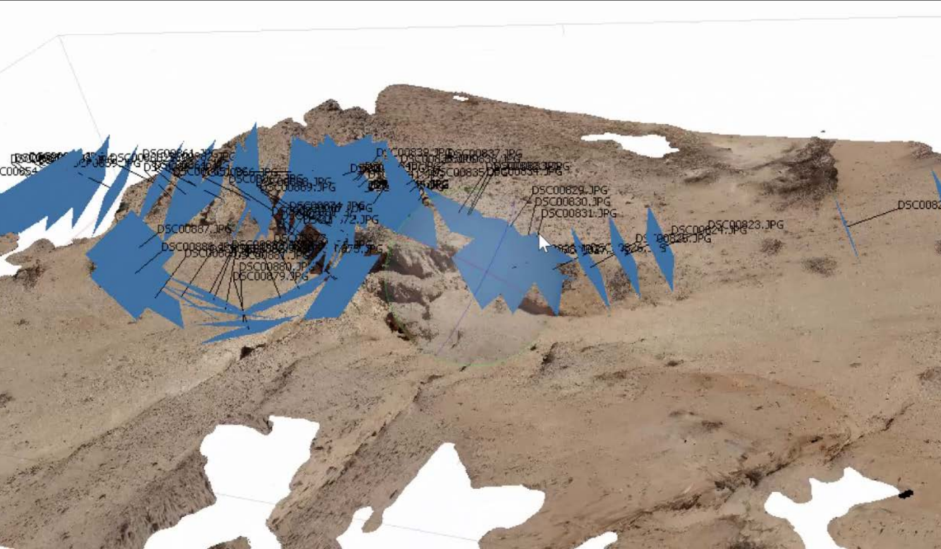
Ground-based structure from motion of Landers fault scarp knickpoint in 2016
